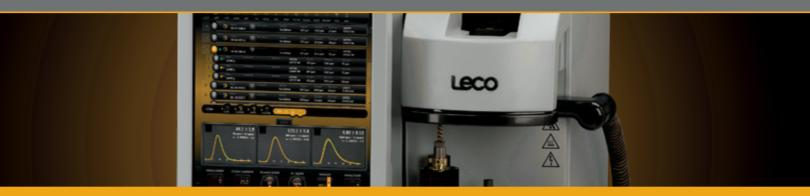
ONH836 Series: Oxygen/Nitrogen/Hydrogen by Fusion
